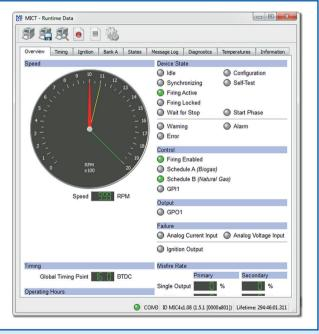
4 For configuration the graphic user interface MICT\* (MOTORTECH Integrated Configuration Tool) is used. Existing configuration files based on the MIC3 series can be used as a reference for setting up a new file for MIC3+ series. The adjustment of individual parameters for new functions or setting ranges may become necessary.
