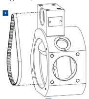
2. Insert the fuel ring 2 through the inlet opening into the drive belt.
