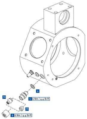
► The gauge ports have been installed.
