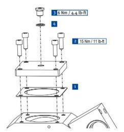
► The closing plate has been installed.
