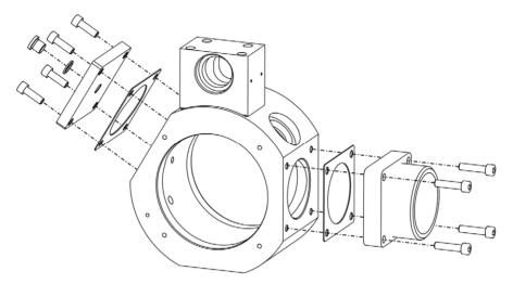
Remove the mounting flange(s) and if necessary the closing plate.
