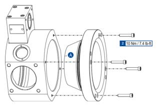
► The outlet nozzle has been installed.
