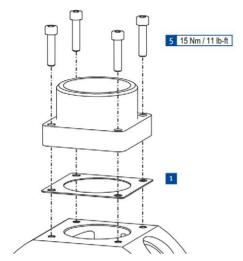
► The mounting flange has been installed.
