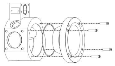
Remove the outlet nozzle and the large O-ring.
